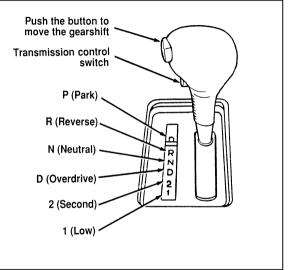
The positions of the console-mounted gearshift
